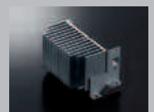
Power Amplifier Board with Aluminum-Extruded Heat Sink
